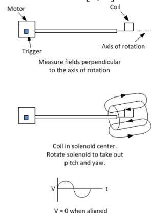
Figure 2: The principle of the center deviation measurement.
