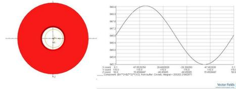
Figure 5: The distribution of magnetic fields in radial direction.
