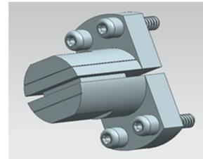
Figure 12: Final design of the groove.
