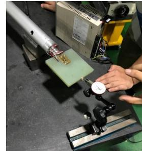
Figure 11: Test the fluctuation of the groove.
