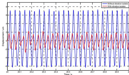
Figure 4: Vibration data of support of bipolar magnet under rated vibration power.
