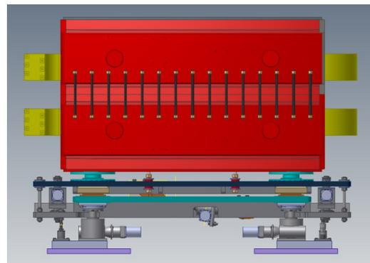
Figure 1: Structure of dipolar girder system with the vibration isolator.
