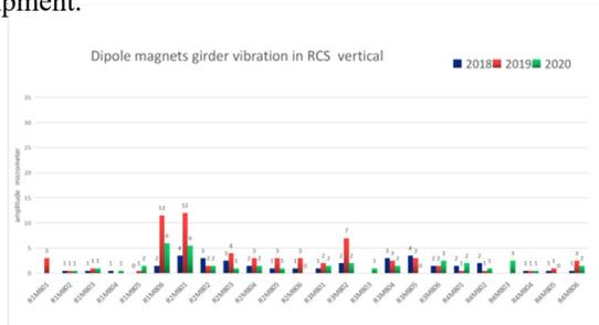
Figure 5: Measurement of long-term vibration of dipole magnet support.
