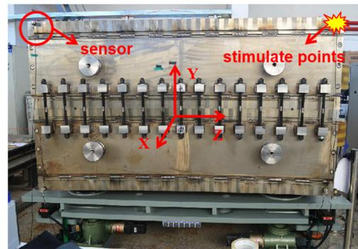
Figure 3: Measurement of long-term vibration of dipole magnet support.
