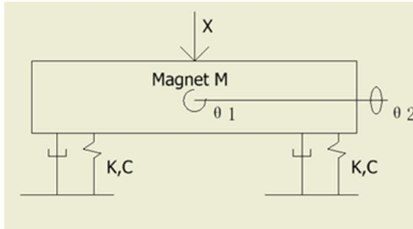
Figure 2: Dynamic model of magnet support system.
