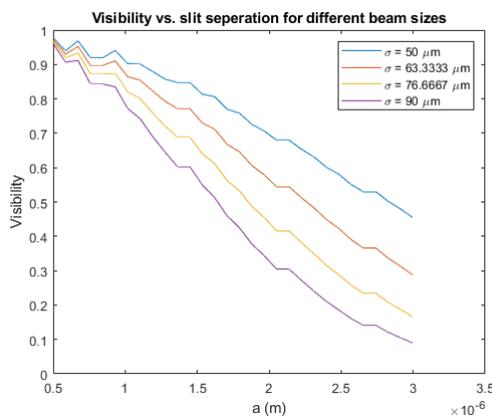
Figure 3: Visibility versus slit separation.
