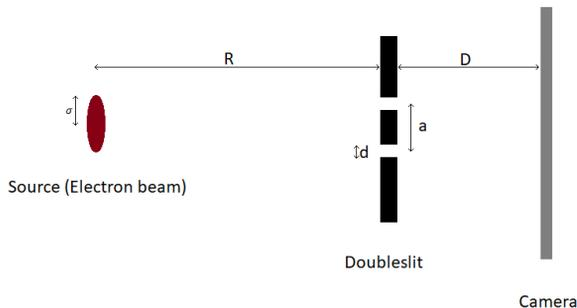
Figure 1: Double slit layout.
