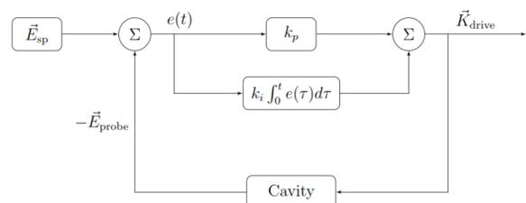
Figure 1: Circuit model of a resonant mode in a cavity [16].
