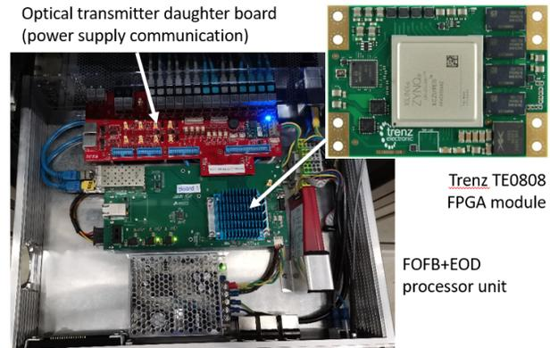
Figure 1: Updated hardware used to implement the FOFB and EOD systems.
