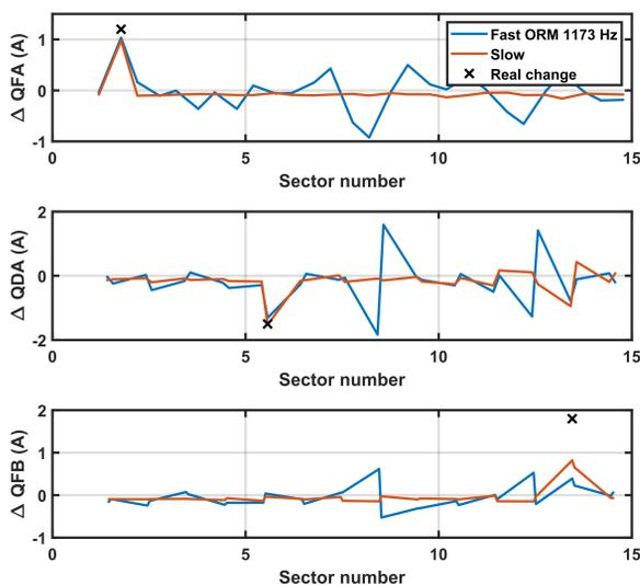
Figure 6: LOCO extracted changes to the quadrupoles using ORMs measured in a serial fashion using fast vs slow methods. Typical QFA, QDA and QFB settings are 139 A, 82 A and 120 A.
