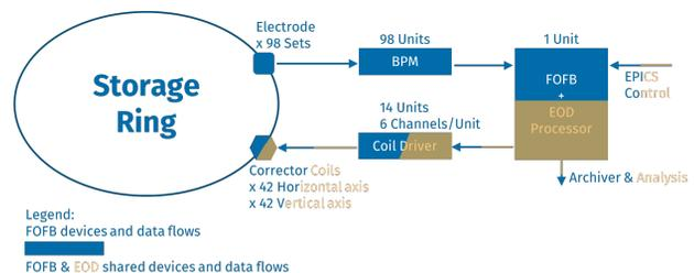
Figure 2: Simplified system architecture and data flows.
