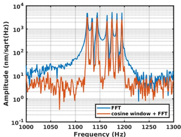
Figure 4: Spectrum of the horizontal position with seven correctors driven simultaneously.
