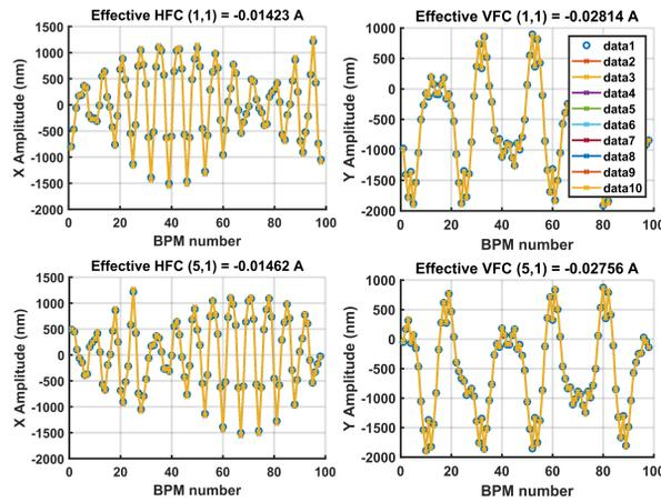
Figure 5: Sample of the closed orbit patterns extracted from the position data. Circles represent expected closed orbits based on a simulated model. The 9 separate data sets indicate repeatable results.
