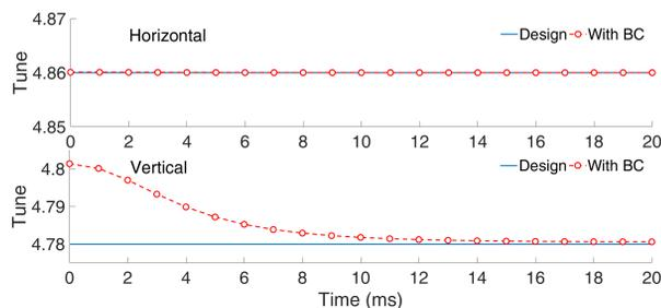
Figure 4: (Color)The tunes in one period with (red dash line with circles) and without (blue solid line) BC bump magnet.
