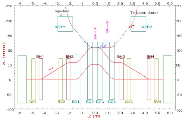
Figure 2: The schematic layout of injection system.
