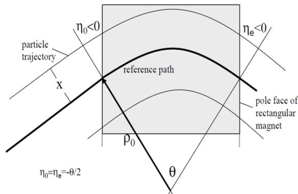
Figure 3: The diagrammatic sketch of the edge focusing.
