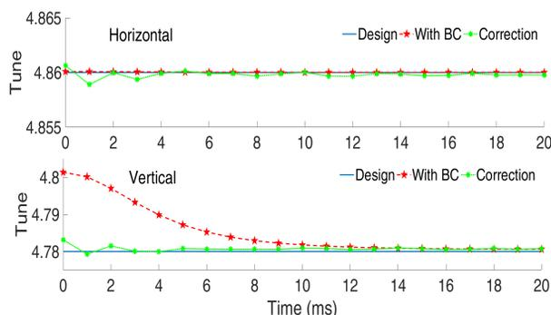
Figure 6: The tunes in one period with (red dash line with pentagram) and without (blue solid line) BC bump magnet compared with the tune after correction (green dot line with asterisk).
