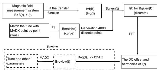
Figure 5: The flow process diagram of the correction of the edge focusing effect.
