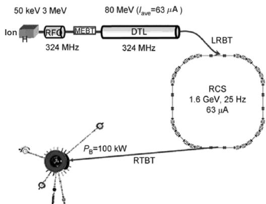
Figure 1: The schematic layout of CSNS.
