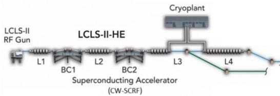
Figure 1: Schematic of the proposed LCLS-II-HE superconducting linac (not to scale).
