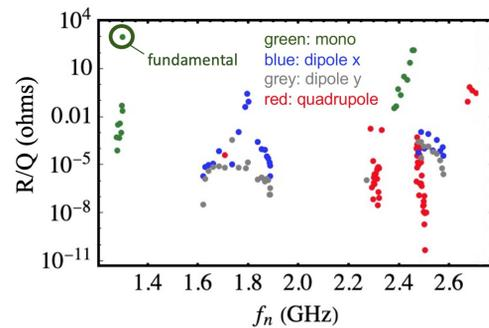
Figure 2: The plot shows simulated transverse R/Q for dipole modes and longitudinal R/Q for monopole modes of the LCLS-II superconducting 1.3 GHz cavity.
