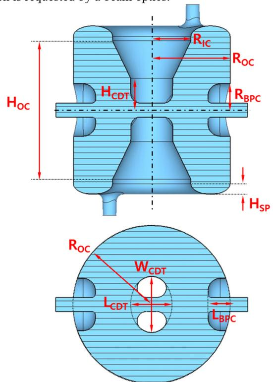
Figure 2: Parametrically designed HWR.
