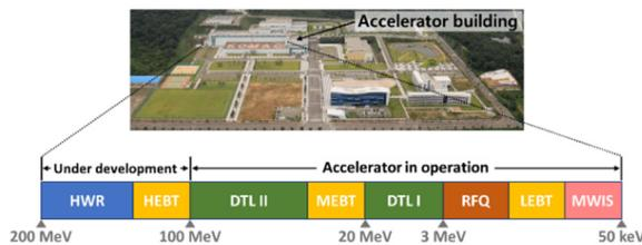
Figure 1: Layout of the proton linac in KOMAC.
