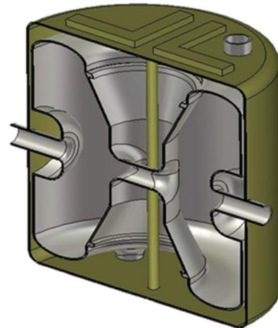
Figure 3: Reinforced design of the cavity and the helium jacket.
