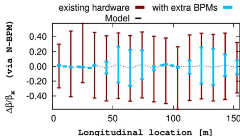
Figure 1:  $\beta$ -beat via N-BPM method for ideal tracking simulations with existing PSB BPMs (red), and with extra BPMs (blue) at optimal  $\Delta\phi$  in periods 1, 2, 3, 10 and 11. Error bars are the systematic uncertainty on the reconstruction.
