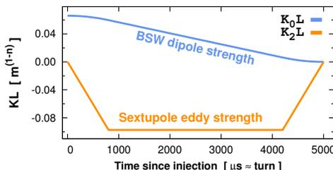
Figure 2: Integrated dipole and sextupole strength during collapse of injection (BSW) orbit bump.
