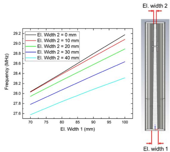
Figure 3: Simulated frequency as function of the electrode width without frequency correction for 32 MHz.
