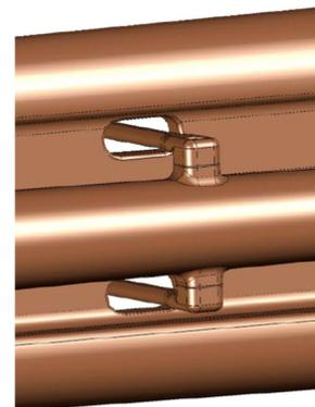
Figure 4: Pair of electrodes with stabilizers and opening in the other electrode pair for the bridging.
