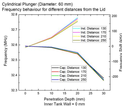
Figure 2: Simulated tuning range for the plungers.
