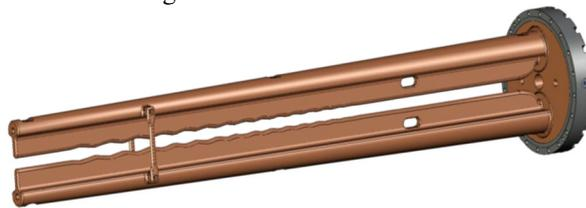
Figure 1: Pair of vanes of the split coaxial RFQ.
