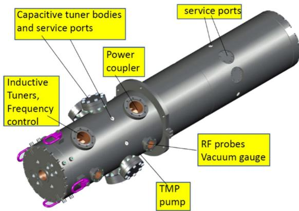
Figure 5: RFQ 3D view and function of flanges.
