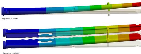
Figure 6: Mechanical quarter wave oscillation modes of the vane pairs at 18 Hz and 25 Hz.
