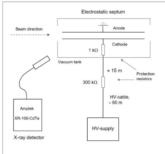
Figure 2: Schematic measurement set-up, with the X-ray detector at the upstream flange of the electrostatic septum.
