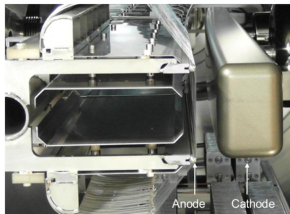
Figure 1: The electrostatic extraction septum in the beam direction with the anode wires and the cathode pointed out. The circulating beam area is to the left, and the extraction channel is to the right between the anode wires and the cathode.
