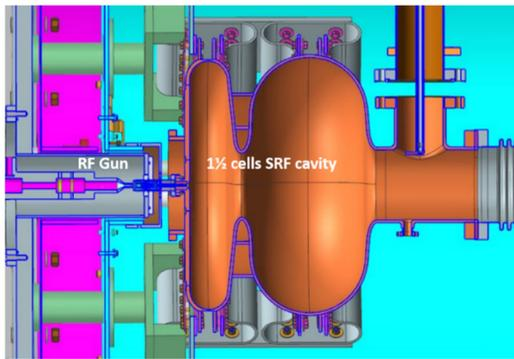
Figure 2: 1 1/2 cells prototype general view.
