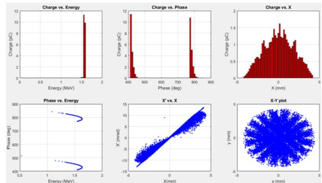
Figure 4: Particle distribution at the exit of the cavity.
