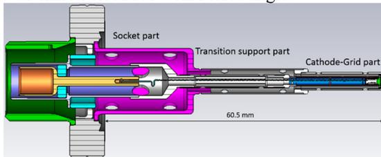
Figure 5: Cross-section of the cathode-grid assembly.
