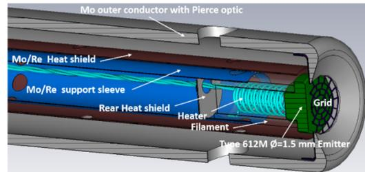
Figure 7: Detailed view of the cathode-grid area.
