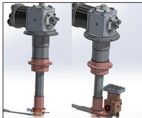
Figure 2: Cryocooler with (left) 5.1 GHz cavity and (right) SLAC cavity.
