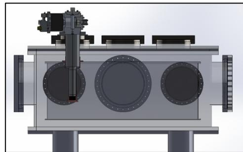
Figure 1: Side view of vacuum chamber with cryocooler and Al thermal shield (shaded).
