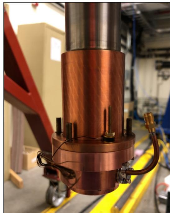
Figure 4: 5.1 GHz cavity mounted on cryocooler.
