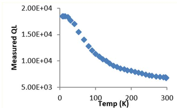
Figure 6:  $Q_L$  for 5.1 GHz cavity vs temperature.
