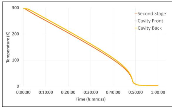
Figure 5: Cooldown curve for 5.1 GHz copper cavity.
