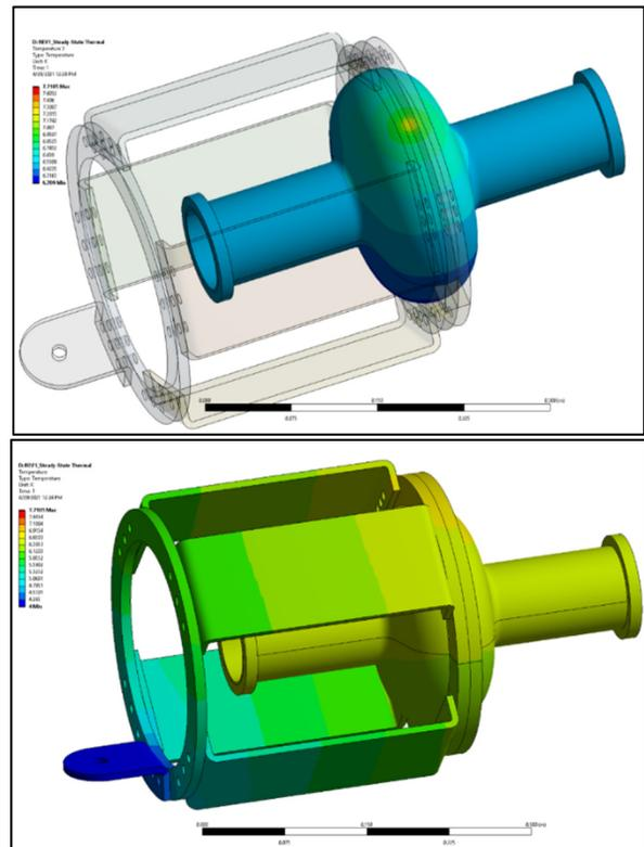
Figure 3: FEA thermal simulations for Nb 1.3 GHz cavity. The yellow dot simulates 1 W of heat on the inner cavity wall.
