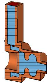
Figure 1: Cross section of the proposed rotationally symmetric RF gun.
