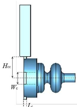
Figure 3: 3D schematic diagram of the RF gun with the coupler.
