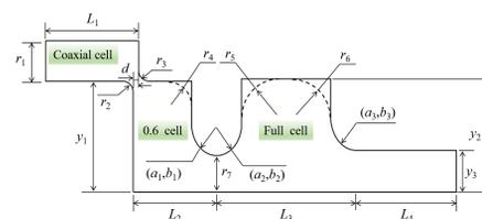
Figure 2: Cross section of the 1.6 cell RF gun (Solid line is the original gun; Dash line is the optimized gun).
