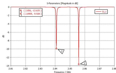
Figure 4:  $S_{11}$  parameter of 0 mode (2) and  $\pi$  mode (1).
