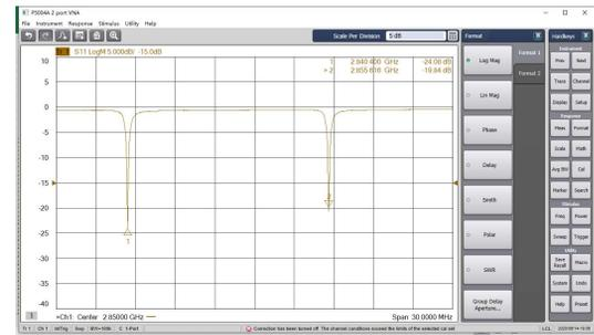
Figure 9: The measurement curve of S11 parameter.
