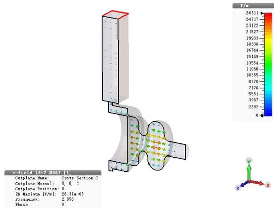
Figure 6: Cross section of the 3D electric field distribution.
