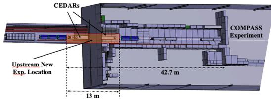
Figure 1: Upstream location of the EHN2 hall in the CERN North Area identified for the new experimental test setups of NA64 $\mu$  and MUonE marked in red, the available 42.7 m space after removal of the beamline elements for the final installation of MUonE and the location of the current COMPASS experiment which will be used for AMBER/NA66.
