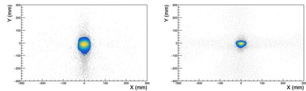
Figure 6: Beam size for a low divergence beam optics –  $\sigma_x = 13$  mm,  $\sigma_y = 22$  mm (left panel) and that for a focused beam optics –  $\sigma_x = 10$  mm,  $\sigma_y = 12$  mm (right panel) from the Gaussian fit of the distributions.
