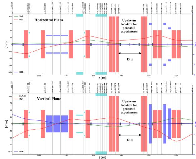
Figure 5: Updated optics option for a small beam with divergence  $< 1.5$  mrad as required by NA64 $\mu$  at the proposed upstream location (the downstream part is not matched). The red, blue and green rays correspond to the transport matrix elements as given by the legends. Red Box – Quadrupoles ; Blue Box – Bends ; Cyan – Collimators.
