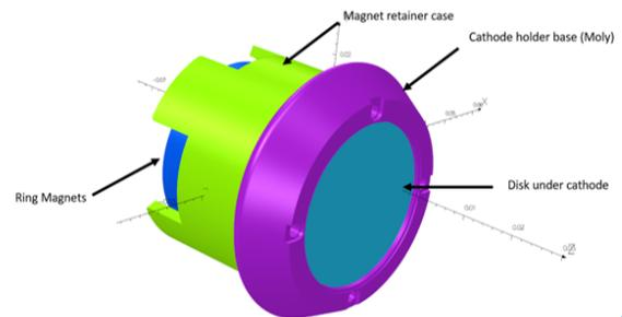
Figure 1: Cathode puck holder with different components.
