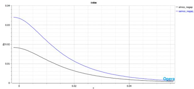
Figure 3: Field distribution along beam axis for different magnets.
