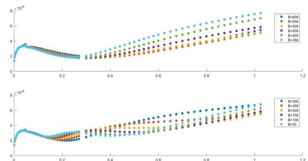
Figure 6: Normalized emittance along beam trajectory for different configuration of magplate and solenoid. B in the legend represents the amount of the field from the magplate, the rest of the field was contributed by the solenoid. Total field on the cathode was kept constant at 600 Gauss for every case.
