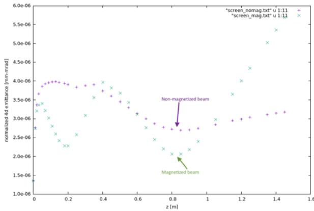
Figure 7: Comparison of magnetized and non-magnetized beam emittance from the same beam parameters. The magnetized beam was generated using the hybrid (magnet+solenoid) method.
