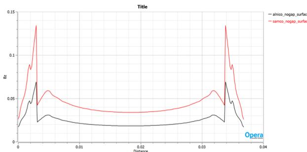
Figure 4: Field profile on the cathode surface for different magnets.
