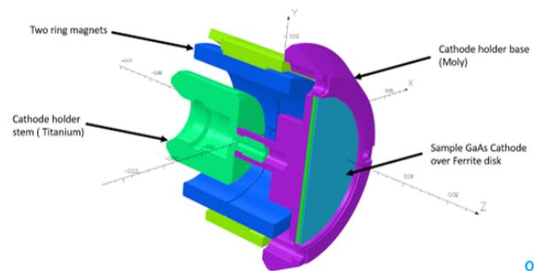
Figure 2: Cross section of the cathode holder, showing the permanent magnet arrangement.
