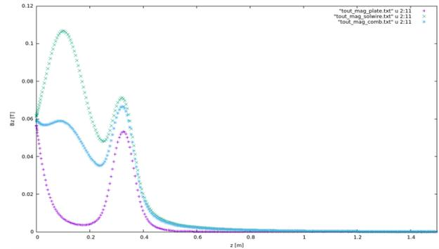
Figure 5: Field profile generated from GPT for different configurations- only magplate, only solenoid and the hybrid magplate+solenoid approach.
