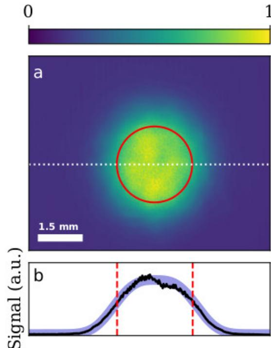
Figure 1: Pump profile. (a) The 1450 nm pump profile measured with an InGaAs SWIR camera. A 3 mm diameter red pupil indicates the clear aperture of the DSTMS crystal. (b) The radial profile in black overlaid on a super-Gaussian profile of order 1.5 (blue) showing good agreement.
