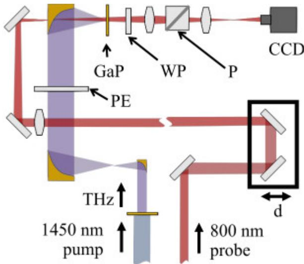
Figure 2: Experimental Setup. An ultrashort 1450 nm pump generates a THz pulse in DSTMS. This THz is relayed to a GaP electro-optic crystal, where it co-propagates with a 30 fs 800 nm probe. The probe is transversely wider than the THz spot at the GaP and its timing with respect to the THz pulse is scanned with a delay line. The probe is imaged through a quarter wave plate (WP) and a polarizer (P) to a CCD.
