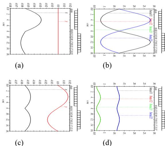
Figure 5: (a) orbit of normal FODO, (b) optics of normal FODO, (c) orbit of skew FODO, (d) optics of skew FODO. A kink of x (horizontal) orbit is due to the rotation of the coordinate system for QD and QF. Second half of x orbit in (a) shows the reverse bend whereas both magnets have normal bend in (c). Vertical orbit oscillation of around  $\pm 20$  mm is induced in the skew FODO.
