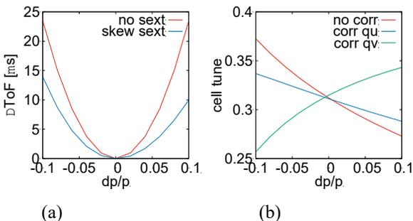
Figure 6: (a) time of flight per cell, (b) red is eigen tune without skew sextupole, green and blue are eigen tune after skew sextuple correction.
