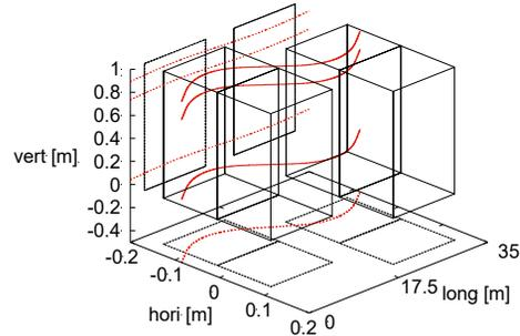
Figure 1: One cell of muon accelerator lattice based on FODO optics. The left block is a defocusing magnet bending the beams in the reverse direction and the right one is a focusing magnet bending in the normal direction. The red curves are orbit at different momenta. The shape of the orbit is the same, but shifts upward when accelerated.
