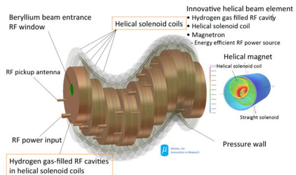
Figure 2: Pictorial drawing of an HCC channel.
