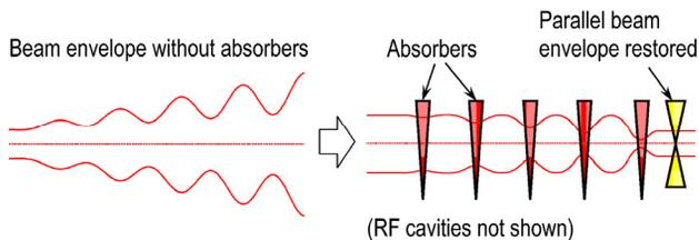
Figure 6: Stabilizing effect of ionization cooling energy absorbers in a channel with a half-integer resonance.
