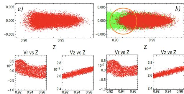
Figure 4: WARP simulations show the plasma lens effect without gas (a) and with gas (b). A red point is an incident particle and a green one is an ionization electron. Only a straight solenoidal magnetic field and RF field are applied, with no dispersion in this simulation. The orange circle shows that the beam is focused by the plasma lens.
