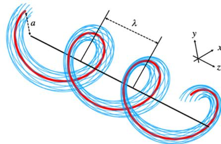
Figure 1: Typical beam paths in a HCC (blue), around a design reference orbit (red).
