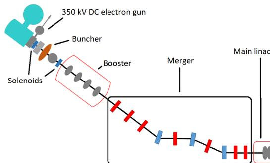
Figure 1: The layout of the injector with an example of a possible merger scheme.
