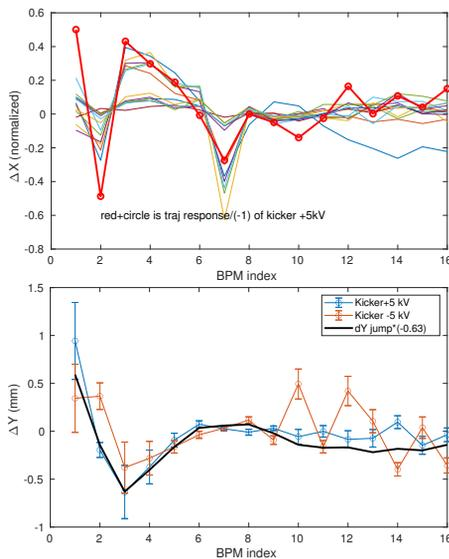
Figure 3: Measured trajectory response of RG1 kicker with  $\pm 5$  kV step changes resembles the trajectory jump pattern measured.
