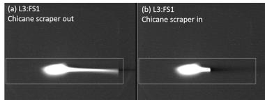
Figure 7: Beam in the middle of chicane on L3:FS1 with horizontal plane indicates energy: (a) with scraper out and (b) with scraper in.
