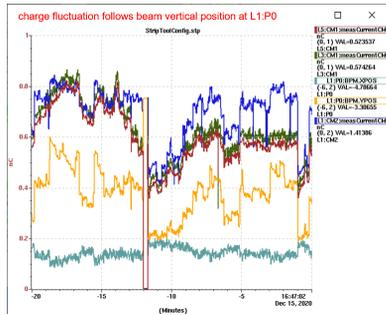
Figure 2: Sudden beam trajectory jumps result in charge loss.
