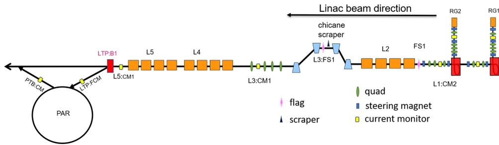
Figure 1: A sketch of the APS linac beamline. Two slots, RG1 and RG2, at the front of the linac, are available for the installation of thermionic rf guns.
