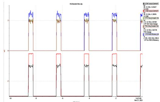
Figure 10: Topup test run with two linac pulses and 2 nC at PTB and 100% linac to PAR injection efficiency.
