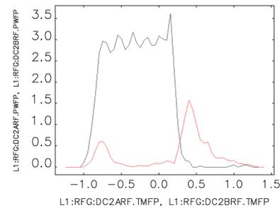
Figure 4: Prototype gun forward (black) and reflected (red) RF waveform.
