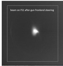
Figure 6: Beam centered on FS1 by adjusting RG2 frontend steering.
