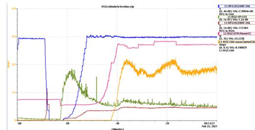
Figure 5: 180 mA gun current was extracted with cathode heater power at 25 W and gun rf power at 3 MW.
