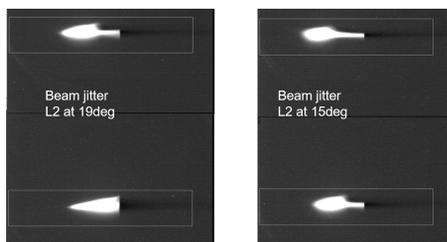
Figure 8: Energy jitter in the middle of chicane as observed on L3:FS1 with horizontal plane indicates energy: (a) jitter before fine phase tuning and (b) jitter after fine phase tuning.
