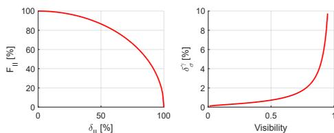
Figure 3: Left: Influence of the intensity imbalance on the measurement visibility. Right: The relative beam size error as a function of visibility for a case with a constant -1% relative visibility error in the system.
