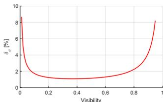
Figure 4: Beam size measurement error as a function of visibility for a given detector sensitivity.
