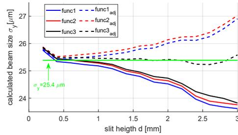
Figure 2: Calculated beam size as a function of the slit opening. The solid lines show the results calculated with the preset aperture separation  $D_y$ ; the dash lines are calculated with the effective separation  $D_y^{eff}$ , different color presents fitting with different functions. The ideal beam size is 25.4  $\mu\text{m}$  (green-line), and the slit separation is 7 mm.
