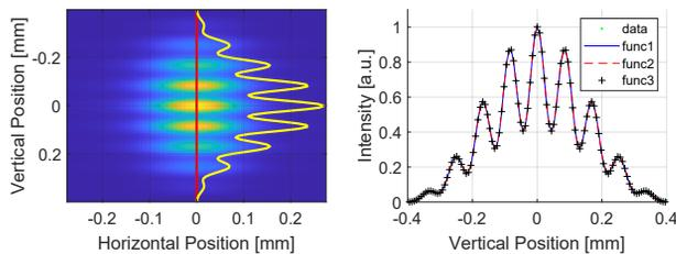
Figure 1: Left: Simulated interference image at the location of the camera using SRW. Right: The normalized intensity distribution (stars) along the vertical center, the lines and crosses are fittings using  $f_1, f_2$ , and  $f_3$  defined in the text.
