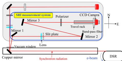
Figure 5: Layout of the SRI measurement system at DSR.
