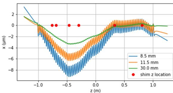
Figure 5: Trajectories of the APS28#12S undulator at 8.5-, 11.5-, and 30-mm gaps before trajectory tuning (6 GeV). The side shim tuning locations are indicated by the red dots.
