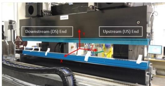
Figure 1: The first APS28 undulator on the measurement bench with the measurement coordinate system overlaid.
