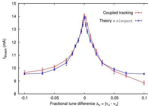
Figure 3: Transverse instability threshold current as a function of fractional tune difference for the full (geometric plus resistive wall) APS-U transverse impedance.
