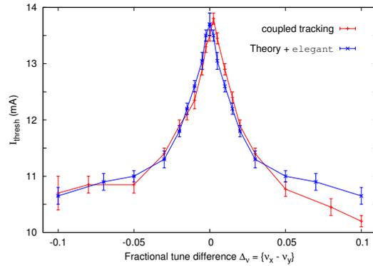
Figure 1: Effect of unequal chromaticities on collective stability near the coupling resonance. Red lines plot the threshold current obtained from the coupled model in elegant, while the blue lines plot the  $I_{\text{thresh}}$  for an uncoupled lattice whose chromaticity is given by the effective value Eq. (12).
