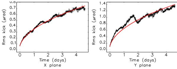
Figure 1: Median time evolution of the rms corrector strength during user operation. Red line shows  $\sqrt{T}$  fit.
