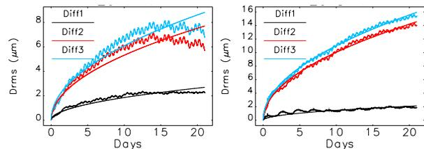
Figure 2: Time evolution of the rms relative displacements of the sensors for two 3-month-long periods. Three values shown are the relative displacements between the three sensors. Square root fits are also shown.
