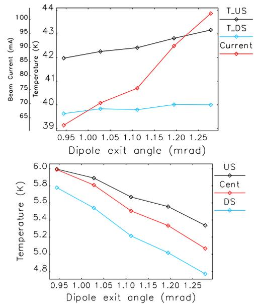
Figure 3: Vacuum chamber temperature (top) and magnet temperature (bottom) as a function of the dipole exit angle. Electron beam current is varied to keep the vacuum chamber temperature approximately constant (also shown on the top plot).
