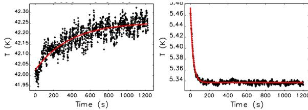
Figure 2: Typical temperature settlement during single scan point measurement. Left – vacuum chamber, right – magnet. Red line shows the exponential fit of the measured (black) points.
