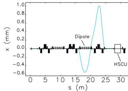
Figure 1: Orbit bump that generates positive orbit angle at the exit of the dipole, which only spans half the sector and has small overall orbit distortion. One lattice sector is shown.
