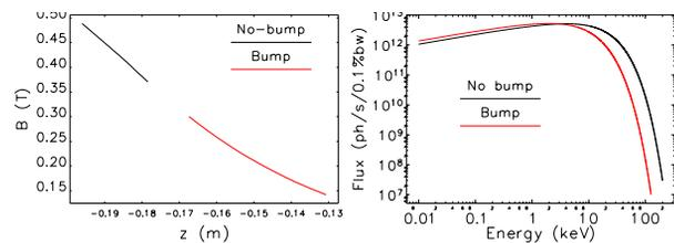
Figure 4: Left: Dipole field along the beam trajectory in the dipole showing only the regions radiating into the HSCU chamber. Right: Photon flux integrated over field regions shown on the left plot.
