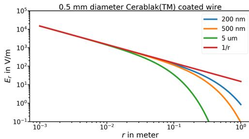
Figure 5: Amplitude of transverse electric field of a Goubau-line using a 0.5 mm diameter copper wire with several thicknesses of Cerablak™ [10] coating at 20 GHz.
