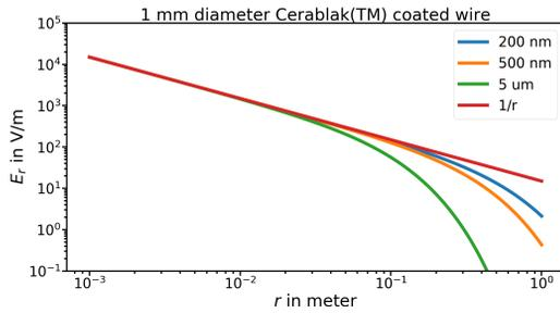
Figure 4: Amplitude of transverse electric field of a Goubau-line using a 1 mm diameter copper wire with several thicknesses of Cerablak™ [10] coating at 20 GHz.
