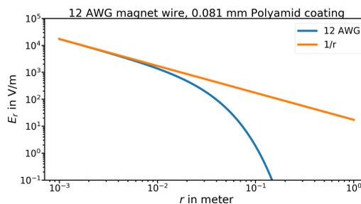
Figure 3: Amplitude of transverse electric field of a Goubau-line using a polyamide coated 12 AWG magnet wire at 20 GHz.
