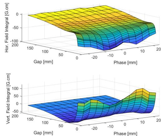
Figure 2: Residual field integrals in both planes of SoftiMAX ID as a function of gap and phase in helical mode.
