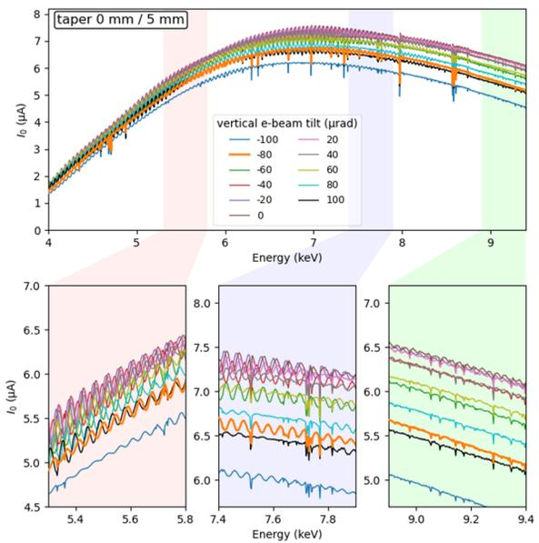
Figure 6: BALDER wiggler spectra at 5 mm gap with zero tapering and different vertical tilt angles of e-beam.
