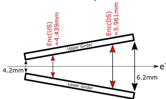
Figure 5: BALDER wiggler taper configuration at minimum gap and maximum tapering with encoders read-outs.
