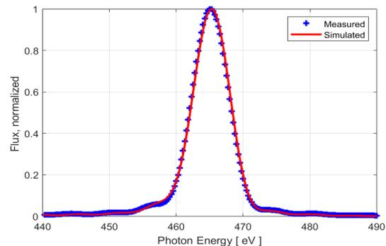
Figure 3: Comparison of simulated and measured SoftiMAX ID spectra at 20 mm gap and zero phase.
