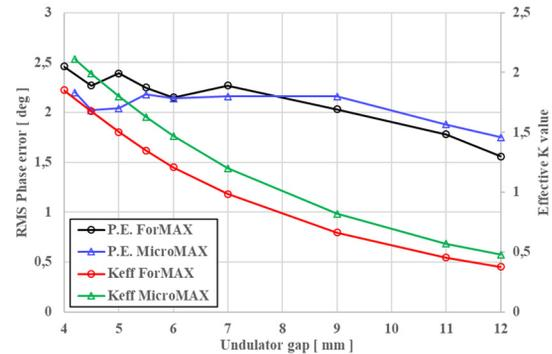
Figure 11: Measured RMS Phase Error (P.E.) and effective K value (Keff) for ForMAX and MicroMAX undulators.
