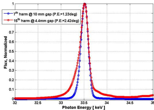
Figure 10: DanMAX spectra of same photon energy from the 7<sup>th</sup> & 15<sup>th</sup> harmonics at 250 mA.
