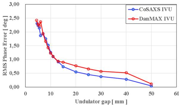
Figure 8: Measured RMS phase error of DanMAX and CoSAXS IVU's prior installation.
