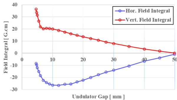
Figure 9: CoSAXS IVU field integrals as seen by the 3 GeV e-beam.
