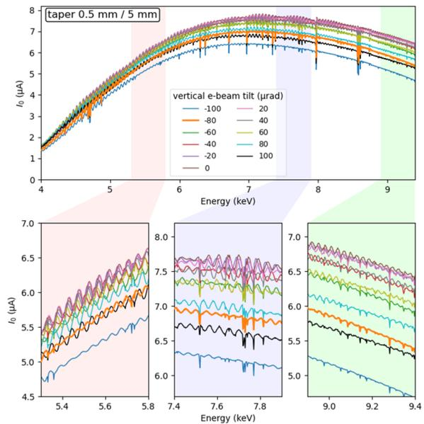
Figure 7: BALDER wiggler spectra at 5 mm gap with 0.5 mm tapering and different vertical tilt angles of e-beam.
