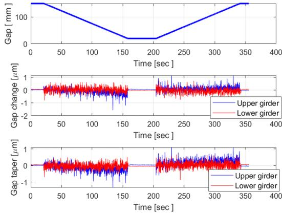
Figure 4: Read-outs of SoftiMAX ID gap and gap tapering while gap movement.
