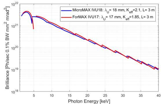
Figure 12: Brilliance estimate of the ForMAX and MicroMAX IVU's at 500 mA beam current.
