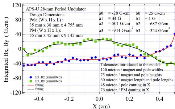
Figure 5: Simulation results of the integrated Bx and By field errors over the length of the APS-U 28-mm model at each different position in X. The "a" and "b" components inserted in the plot represent the integrated field errors of  $B_x$  and  $B_y$ , respectively.
