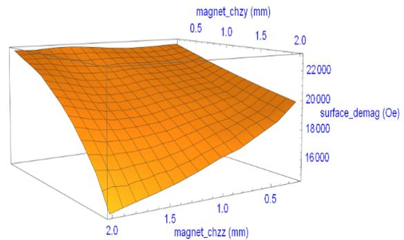
Figure 3: The maximum PM surface demagnetization field of the APS-U 28-mm period undulator design as a function of the PM-zz and -zy chamfers size at a gap of 8.5 mm.
