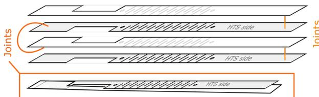
Figure 5: Schematics of the zig-zag soldered tape stack with both facing joints (on the right) and interwoven joints (on the left and bottom sketch).
