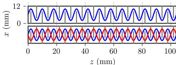
Figure 1: Top: Simplified sinusoidal line current model in the meander-structured tape. Bottom: sinusoidal current in the meander structure (blue line) and a second tape's current with phase shift of  $\lambda_u/2$  and inverse current direction (red line), together forming small current loops in alternating direction.
