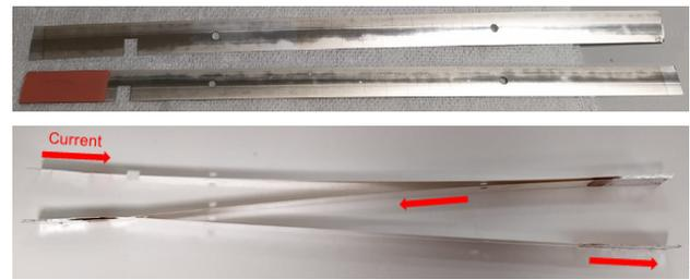
Figure 6: Top: Structured tape piece with a length of 25 cm and the copper-plated tape end. Bottom: tape stack from three HTS tapes, including both types of joints.
