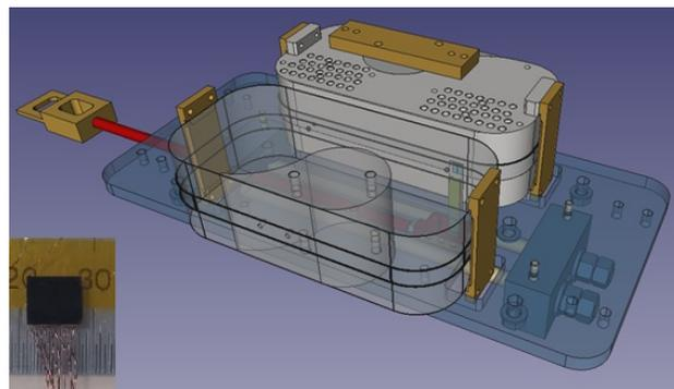
Figure 4: Setup for first field measurements of the single-wound winding formers in the CASPER I liquid helium bath cryostat at KIT. On the bottom left, a Hall-probe array with ten integrated probes is shown.
