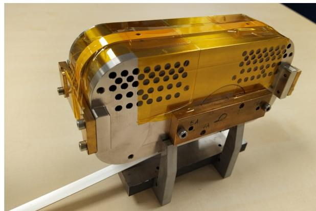
Figure 3: Prototype winding former with structured tape wound according to the jointless winding scheme as described in [4].
