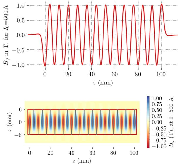
Figure 2: Simulated magnetic field  $B_y$  along the nominal beam axis  $z$  (top) and in the  $xz$ -plane (bottom) in the center of the magnetic gap, i.e. both with a distance of 2 mm to the tape stacks. The parameters used in this simulation are shown in Table 1.
