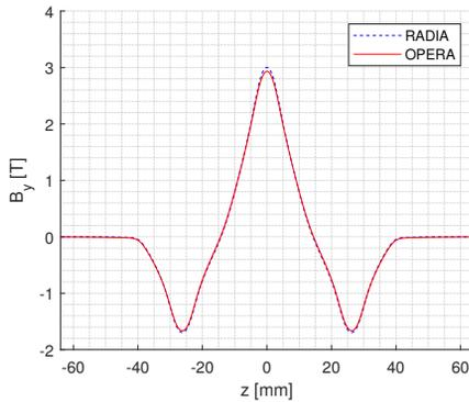
Figure 3: Projection of the magnetic field along the Y axis along the Z longitudinal direction simulated in Radia and Opera-3d.
