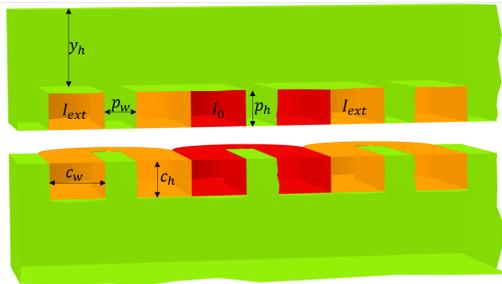
Figure 2: Geometry of the phase shifter.
