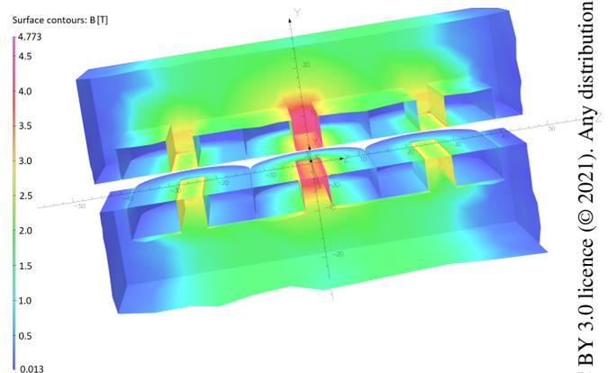
Figure 7: Magnetic field on the phase shifter from OPERA-3d simulation.
