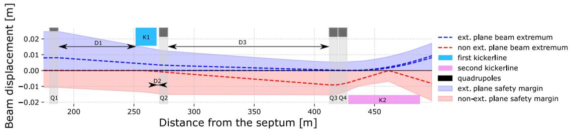
Figure 3: Optimized baseline layout for kicker voltage  $V_0=20$  kV and tunnel length  $l_t=2$  km. The dashed lines show the beam trajectories associated with the maximum excursion of the dilution pattern, and the shaded zones indicate the beam stay clear distance around these trajectories.
