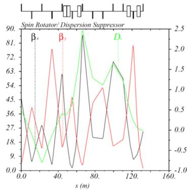
Figure 3: The geometric matching section for the spin rotators. This is coming out of the positive bending arc.
