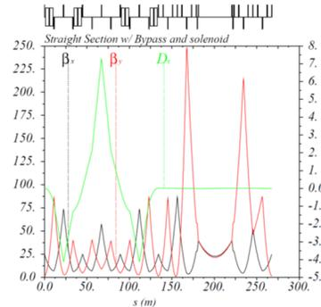
Figure 5: This is the other straight section with the bypass chicane upstream of the solenoid.
