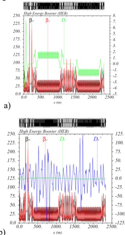
Figure 6: In a) we see the lattice with only the linear dispersions, and in b) we see the nonlinear dispersions.
