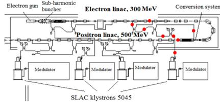
Figure 4: Linac RF measurement points layout.
