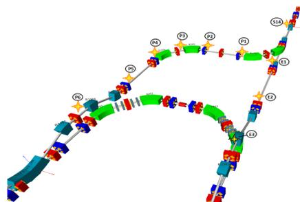
Figure 3: Proposed beam position monitors placing.
