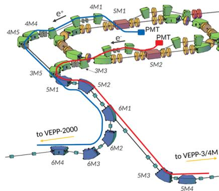
Figure 2: Beam loss monitor layout.
