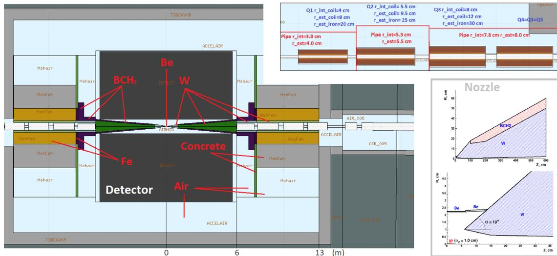
Figure 1: MC interaction region. The passive elements, the nozzles and the pipe around the interaction point are constituted by iron (Fe), borated polyethylene (BCH<sub>2</sub>), berillium (Be), tungsten (W) and concrete. The detector volume is a 11.28 m long cylinder of 6.3 m outer radius with an inner hole of 60 cm radius. The bunker is a 9 m radius and 26 m long cylinder. Top right: IR quadrupoles specifications. Bottom right: detailed description of the nozzle from [7].
