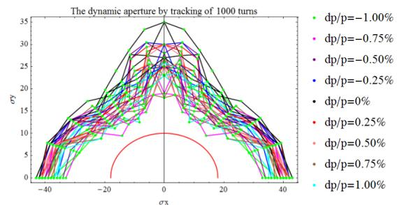
Figure 4: The optimized dynamic aperture for the electron ring.
