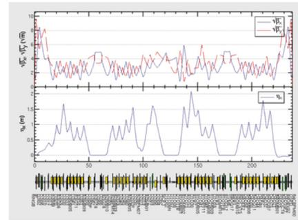
Figure 3: The re-matched beam envelope and dispersion function of the whole ring for the electron ring.
