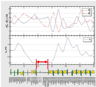
Figure 2: The re-matched beam envelope and dispersion function at the RF region for the electron ring.
