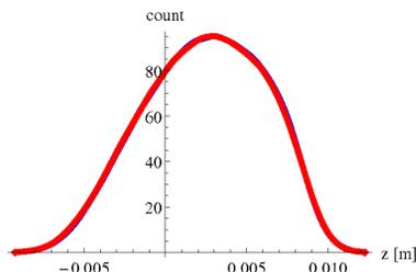
Figure 1: Longitudinal distribution (collision off) obtained using Elegant and IBB considering longitudinal impedance.
