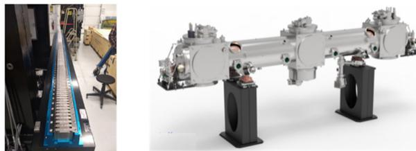
Figure 10: HPMU monokeeper (left) and SCU cryomodule. (right).
