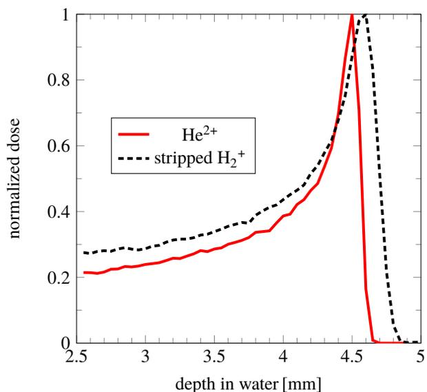
Figure 2: Measured depth-dose profiles in water, normalized to the same peak dose.
