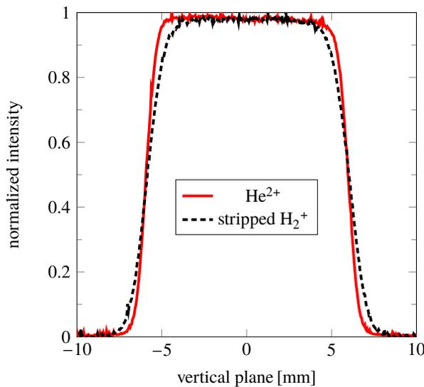
Figure 3: Vertical profile of the central cross-section of the delivered beams.
