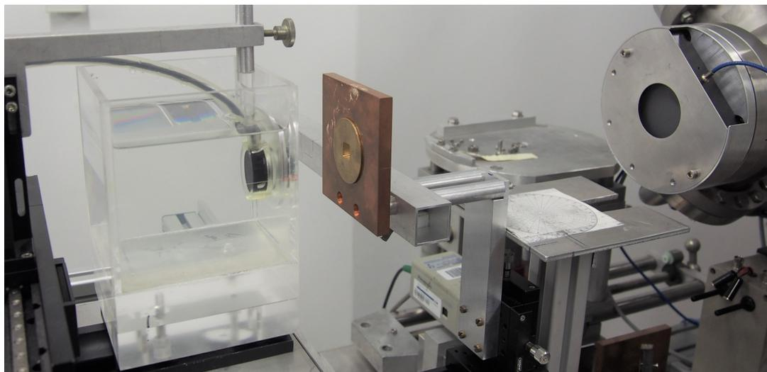
Figure 1: Photo of the common irradiation nozzle. The ions travel from right (vacuum beamline exit port) to left (dose detector in water phantom) in air, while passing through a square brass collimator. The water phantom can be replaced by a CCD camera.
