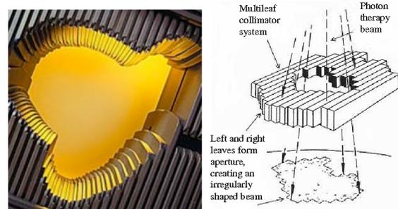
Figure 1: Multi-Leaf Collimator Photograph (left) and schematic depicting an MLC's function (right).
