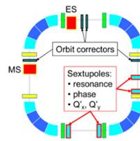
Figure 2: Layout of the superconducting synchrotron.
