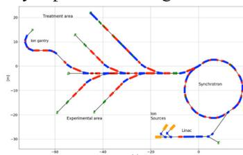
Figure 1: Layout of the synchrotron-based facility.
