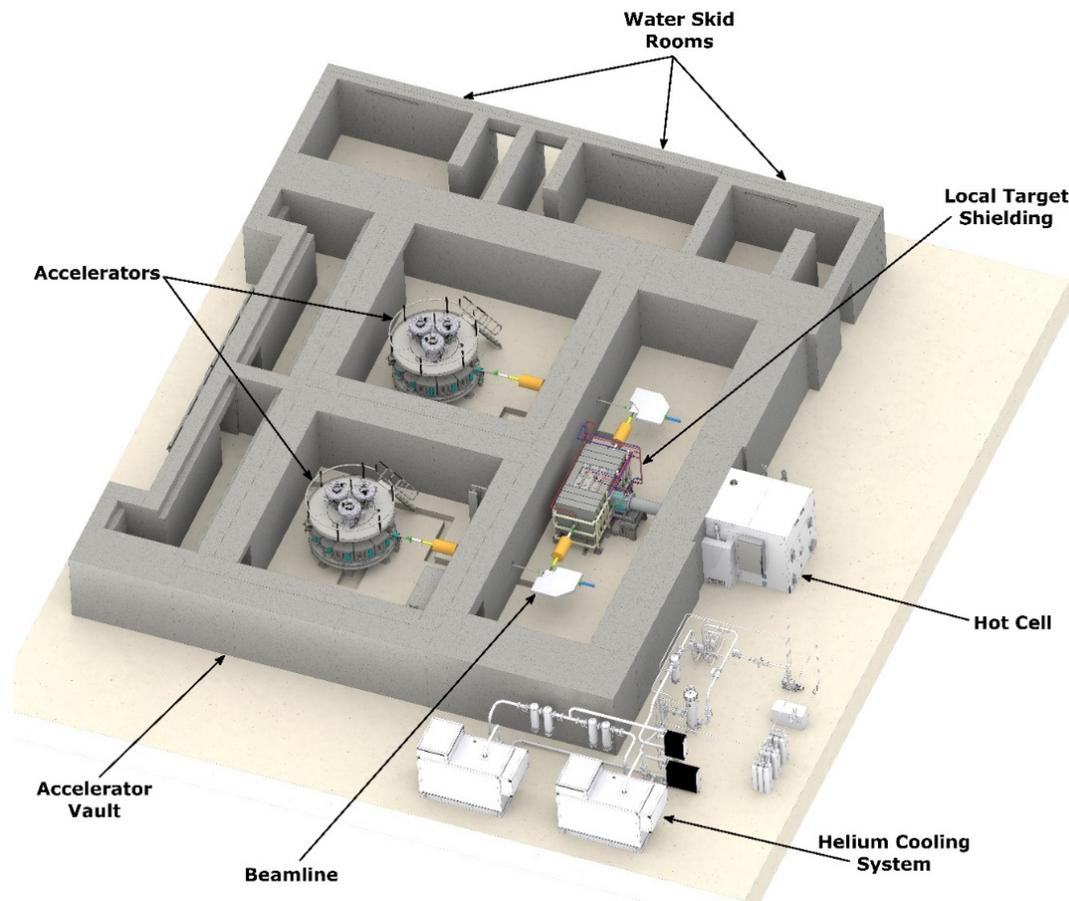
Figure 1: Rendering of the process space of NMR's irradiation facility that will use accelerators to produce Mo-99.
