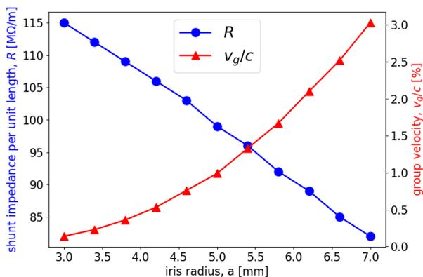
Figure 4: Preliminary results for Shunt impedance and group velocity for single TW cell.
