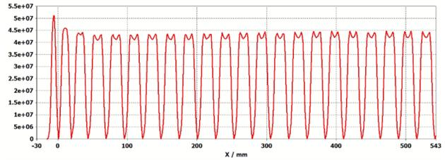
Figure 3: Injector's on-axis electric field.
