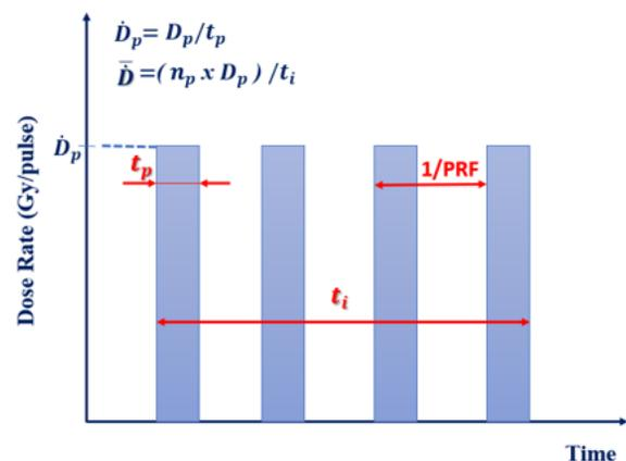
Figure 1: Scheme of an ideal pulsed beam temporal structure.
