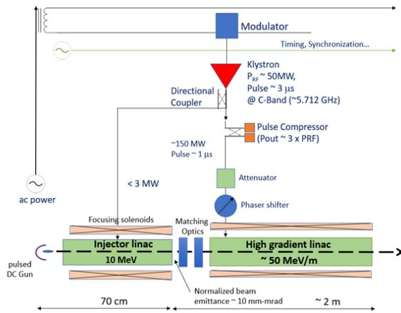
Figure 2: Layout of the C-band accelerator for VHEE FLASH radiotherapy.
