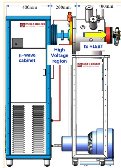
Figure 1: The mechanical view of the proton injector.
