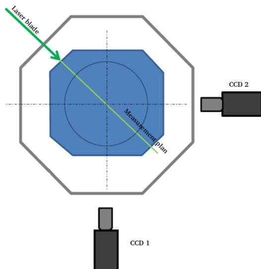
Figure 1: Schematisation of our PIV experimental set up.
