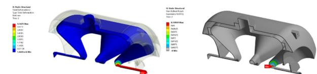
Figure 3: Deformation and plastic strains after applying a tensile force of 7000N on the MYRRHA cavity.
