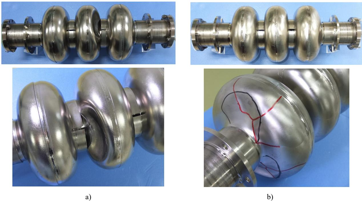
Figure 2: Cavities after deformation. a) Fine grain. b) Large grain (Grain boundary and area of deformation are traced by red and black felt pen, respectively).
