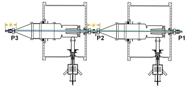
Figure 3: The layout of cavity string. Beam passes right to left through the cavity string.
