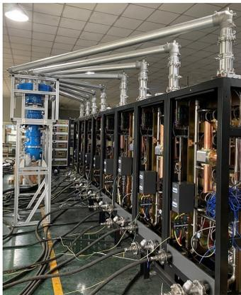
Figure 5: 166.6 MHz 260 kW solid-state amplifier.
