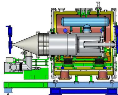
Figure 3: 166.6 MHz SRF cavity module.
