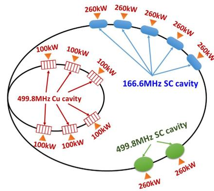
Figure 1: Layout of the HEPS RF system.
