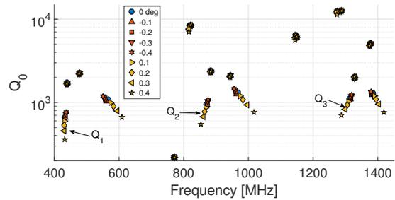
Figure 7: Quality factor vs. Frequency of the QPR at room temperature with a rotation of the rods around the  $y$ -axis with an angle  $\theta$  between  $-0.4^\circ$  and  $0.4^\circ$ .
