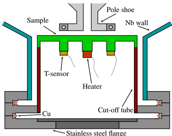
Figure 2: Cross-sectional view of the calorimetry chamber.
