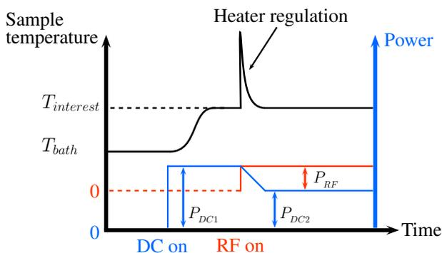
Figure 3: Illustration of the calorimetric measurement principle [2].
